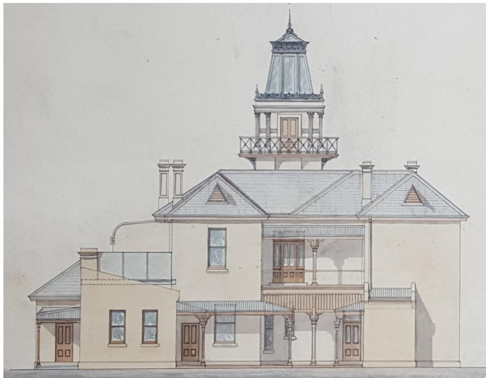
Figure 10: Rowe and Green, 'Plans of Villa for A. Harber Esq. Note the water tanks on the roof to the left hand side.
